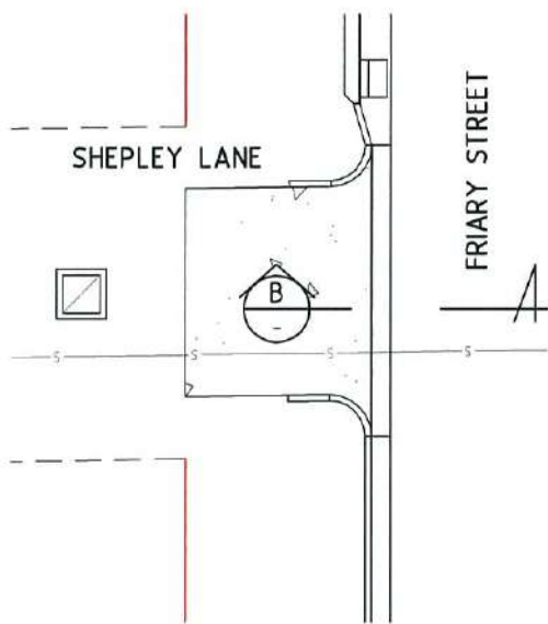
SECTION B TYPICAL LANEWAY CROSSOVER DETAIL SCALE 1:20
