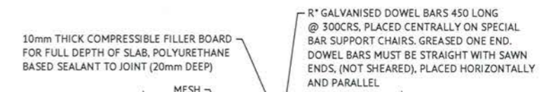
CONTRACTION JOINT (CJ) SCALE 1:10 NOTE: MAXIMUM JOINT SPACING 15.0m R* = R16 FOR SLAB THICKNESS (100mm-150mm) R* = R20 FOR SLAB THICKNESS (151mm-190mm) R* = R24 FOR SLAB THICKNESS (191mm-240mm)
